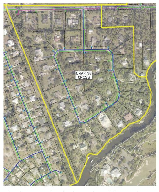
comprise the majority of lots, do not have water service. There is an existing ten-inch water main located on the north side of Broadway Avenue West. There is no gravity sewer in this area, but GIS shows an eight-inch force main located on the north side of Broadway Avenue West.
