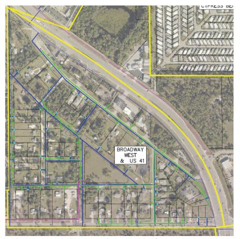
service. There is an existing ten-inch water main located on the south side of Broadway Avenue West and a twelve-inch water main along the west side on US 41. There is no gravity sewer in this area, but GIS shows an eight-inch force main located approximately 1,575 feet to the west of where the force main from this area would connect.
