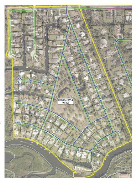
The current layout for this area includes a shared master manhole, pump station, and force main with Charing Cross. Both systems will connect to the existing eight-inch force main. These shared costs have been broken out and prorated based on lots served. The Broadway West's proportion of the shared costs is 80%.
